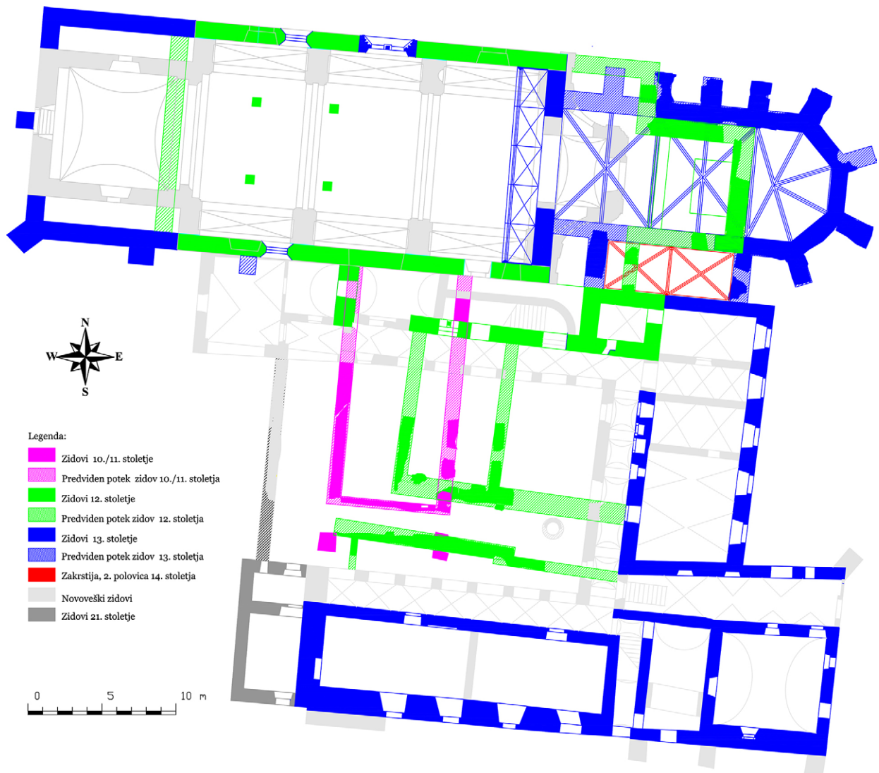
Slika/ Figure 7 Gradbene faze Minoritskega samostana in pripadajoče cerkve po B. Vnuku (Vnuk 2015, tabela X/I). / Construction phases of the Minorite monastery and the associated church after B. Vnuk (Vnuk 2015, Plate X/I).
