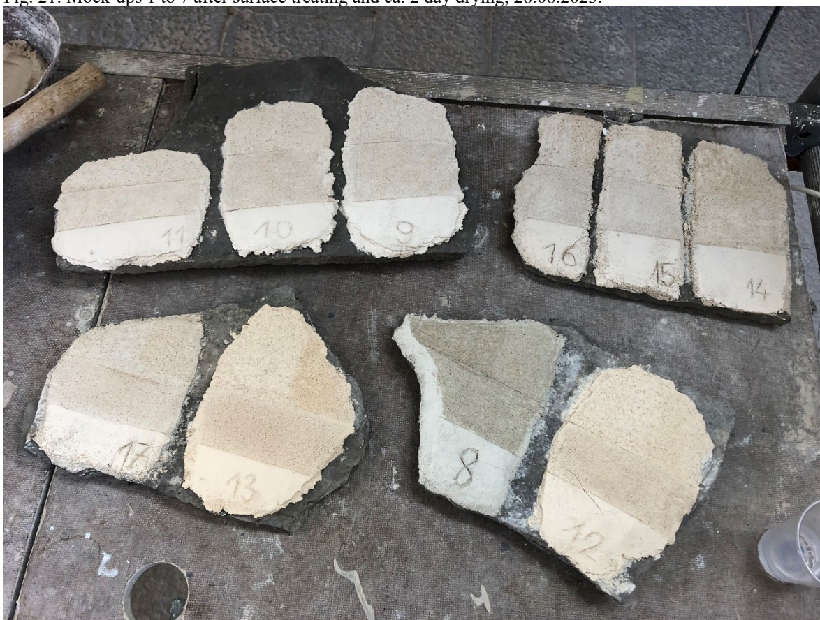
Fig. 22: Mock-ups 8 to 17 after surface treating and ca. 3 day drying; 03.09.2023.
