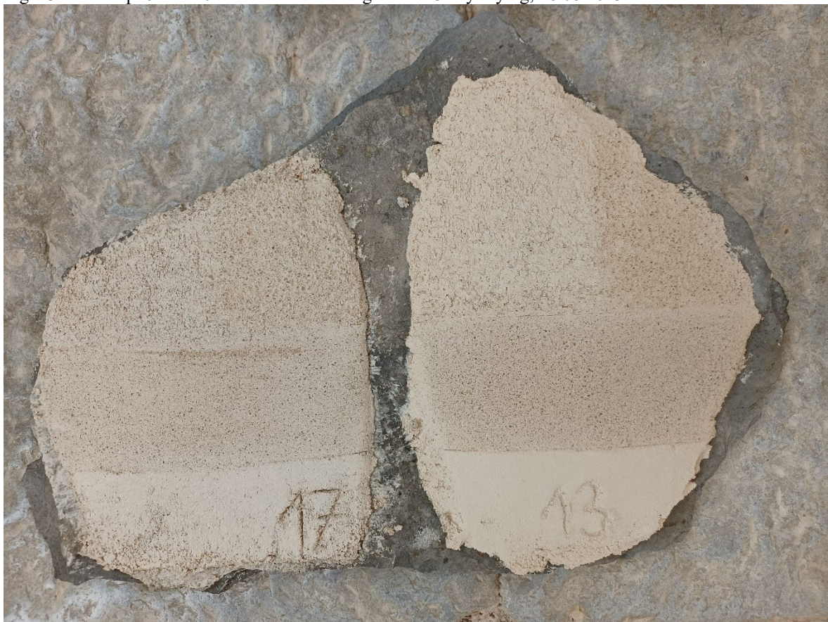
Fig. 24: Mock-ups 13 and 17 after surface treating and ca. 3 day drying; 03.09.2023.
