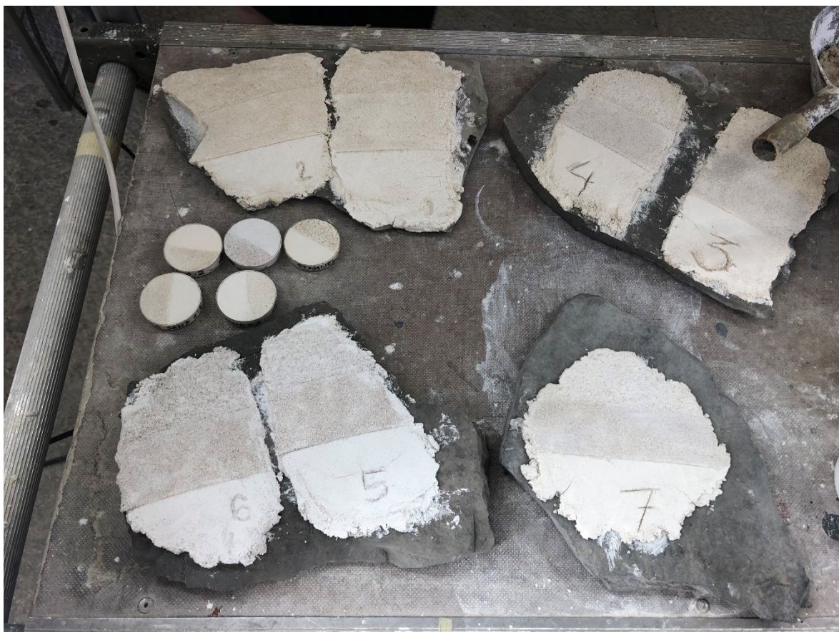
Fig. 21: Mock-ups 1 to 7 after surface treating and ca. 2 day drying; 28.08.2023.
