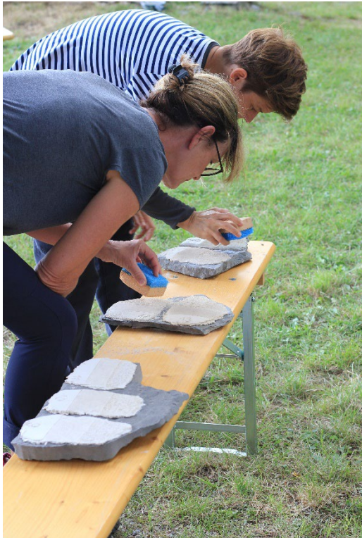
Fig. 20: Treating of mock-ups mortar surfaces; 26.08.2023.
