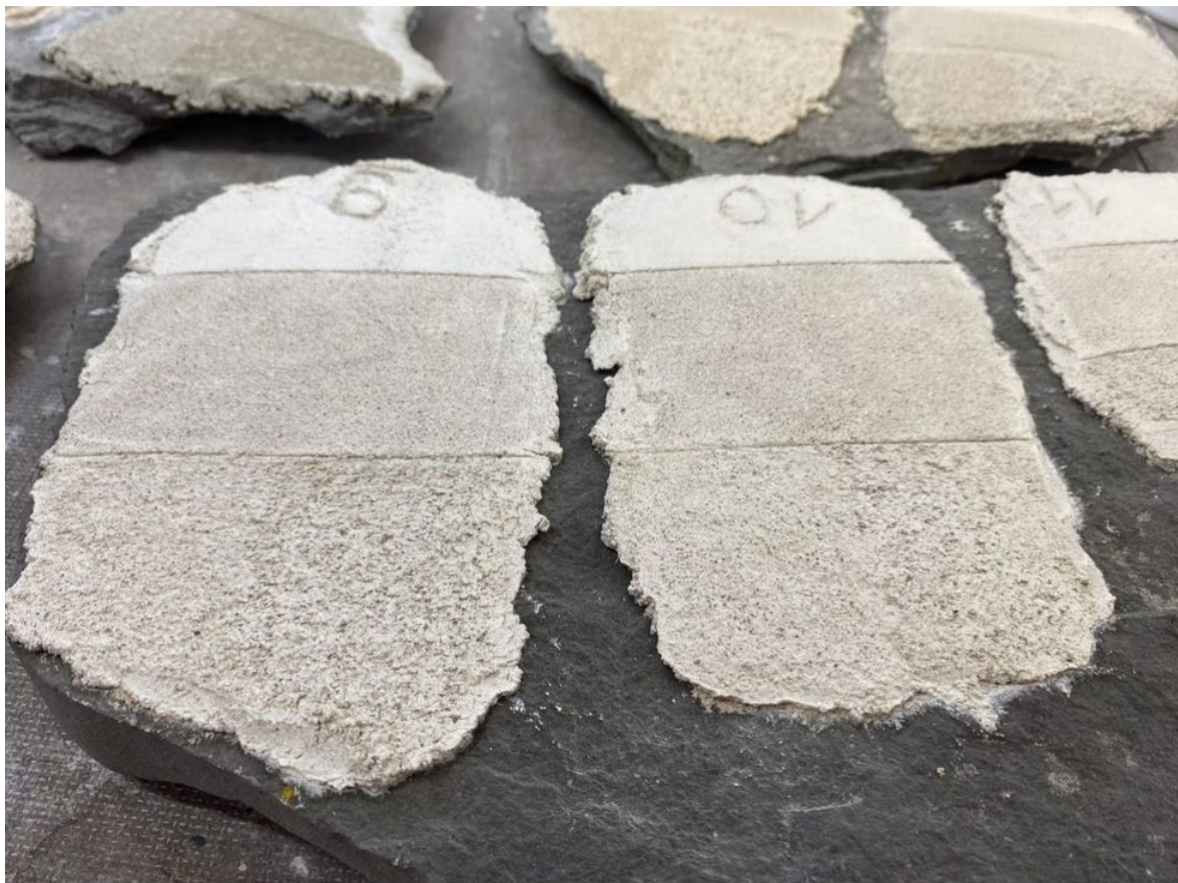
Fig. 23: Mock-ups 9 and 10 after surface treating and ca. 3 day drying; 28.08.2023.
