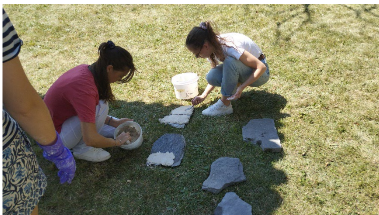
Fig. 19: Applying test mortars on flat limestones; 26.08.2023.
